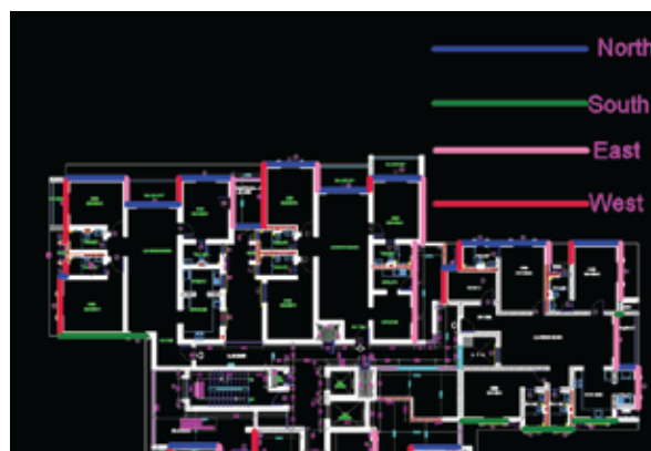
Figure 1: Calculation of orientation wise envelope lengths
