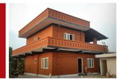
Wienerberger's Porotherm FB Exteria bricks are available in two formats – 200 mm and 150 mm width; these plain-finished bricks have deep grooves only on the top & bottom. These bricks specifically cater exposed masonry requirements for individual houses, commercial buildings and educational institutions - preferably in terracotta finish.
