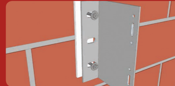
Anchoring the wall brackets
